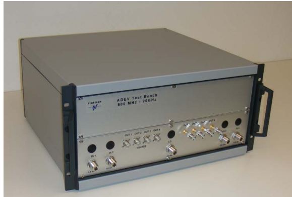
Figure 6. Down-Converter 500MHz - 20GHz
